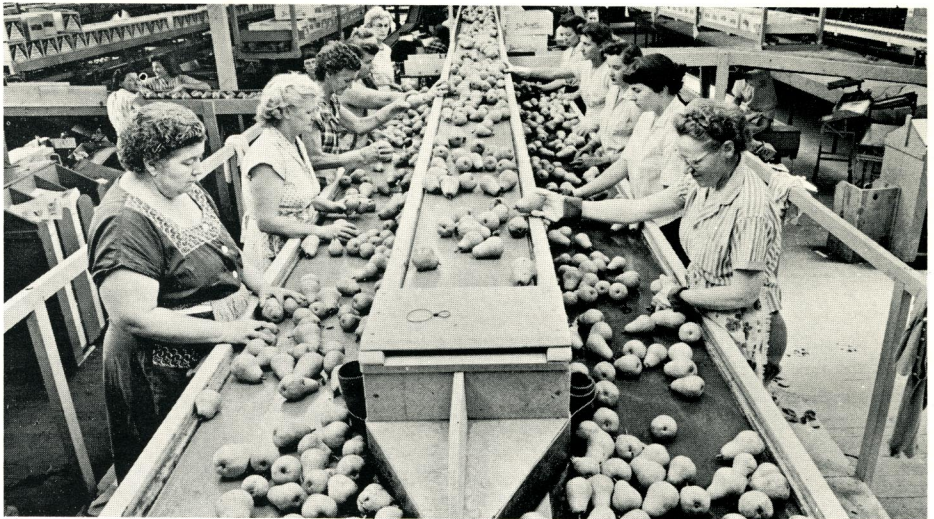
Before packing, freshly harvested pears are carefully graded in the packing house at the New England orchard. Defective pears are removed from the line on the elevated center belt.
